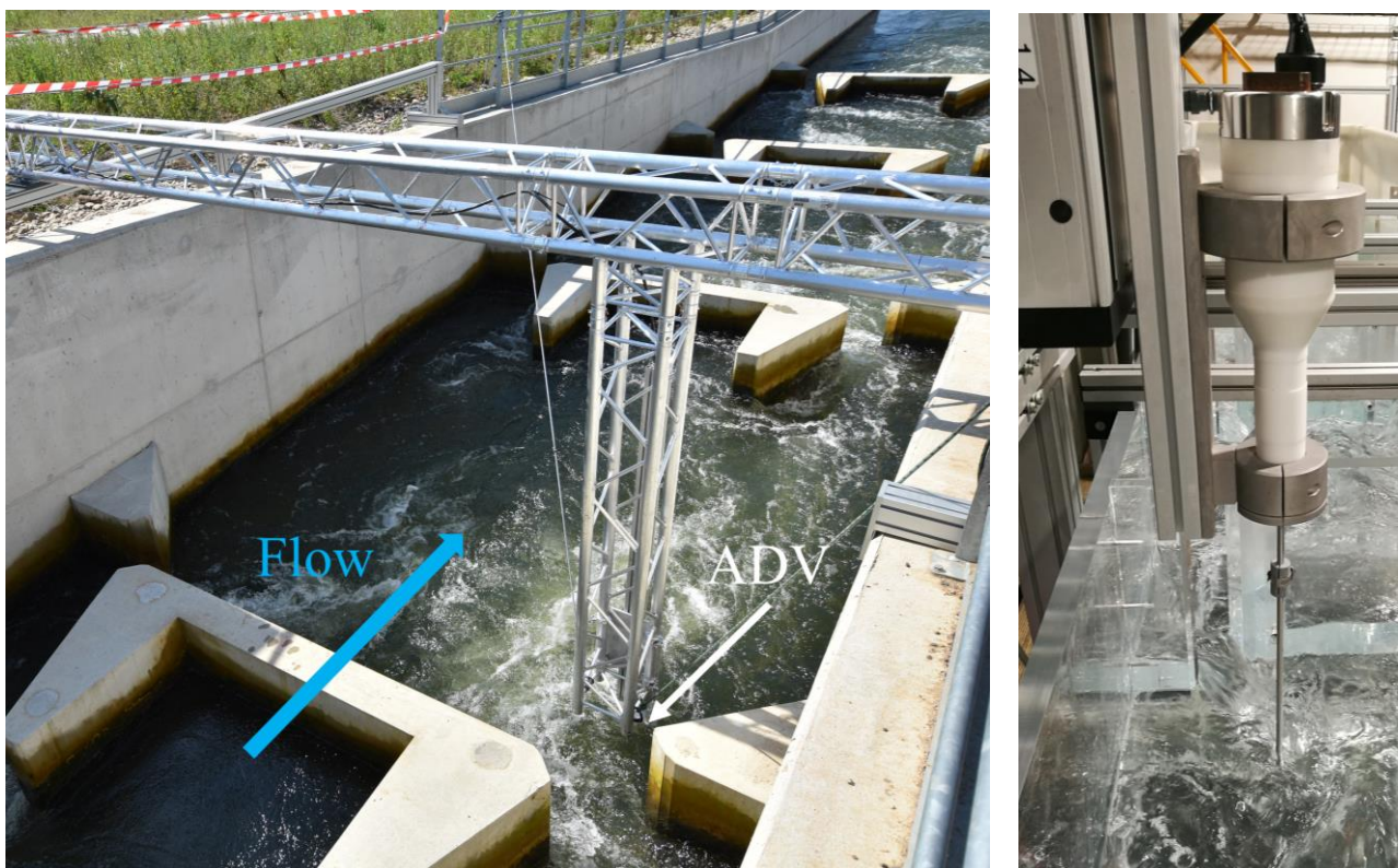
Figure 1. Experimental set-up for (a) the full-scale ADV measurements (Vertical Double Slot Fishway of Malause, Garonne River, France) (b) the 1:6 scale model ADV measurements (Pprime Institute, University of Poitiers, France)
